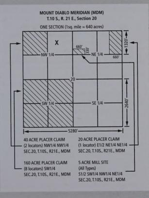
Figure 2. Drawing of a section of land showing different sizes of placer mining claims and a mill site. The legal description method is based on the Public Land Survey System.
